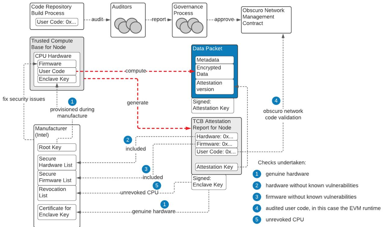
A signature from the EK attests that a signed data packet originates from a genuine CPU. That is not enough for the output of typical confidential computing use cases, as clients have to know what program runs inside the CPU and what firmware.
