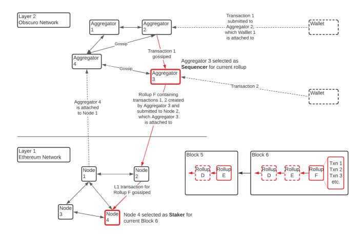
On the bottom right, this diagram also depicts the state of a simple rollup chain as it is found in the sequential L1 blocks.
