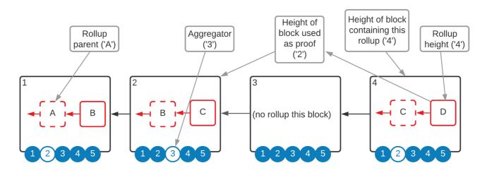
The notation is the following: R\$Rollup\_Height[\$Aggregator, L1\_Proof\_Height, L1\_Block\_Height, \$Nonce]\_.
